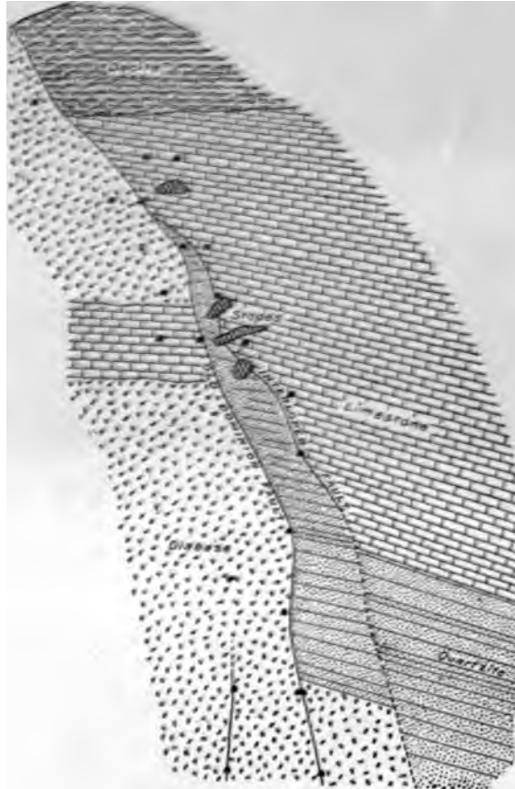
FIG. 117 — VERTICAL SECTION OF THE OLD DOMINION MINE, SHOWING THE OCCURRENCE OF FAULT IN THE DIABASE OF THE FOOTWALL. (RANSOME)
